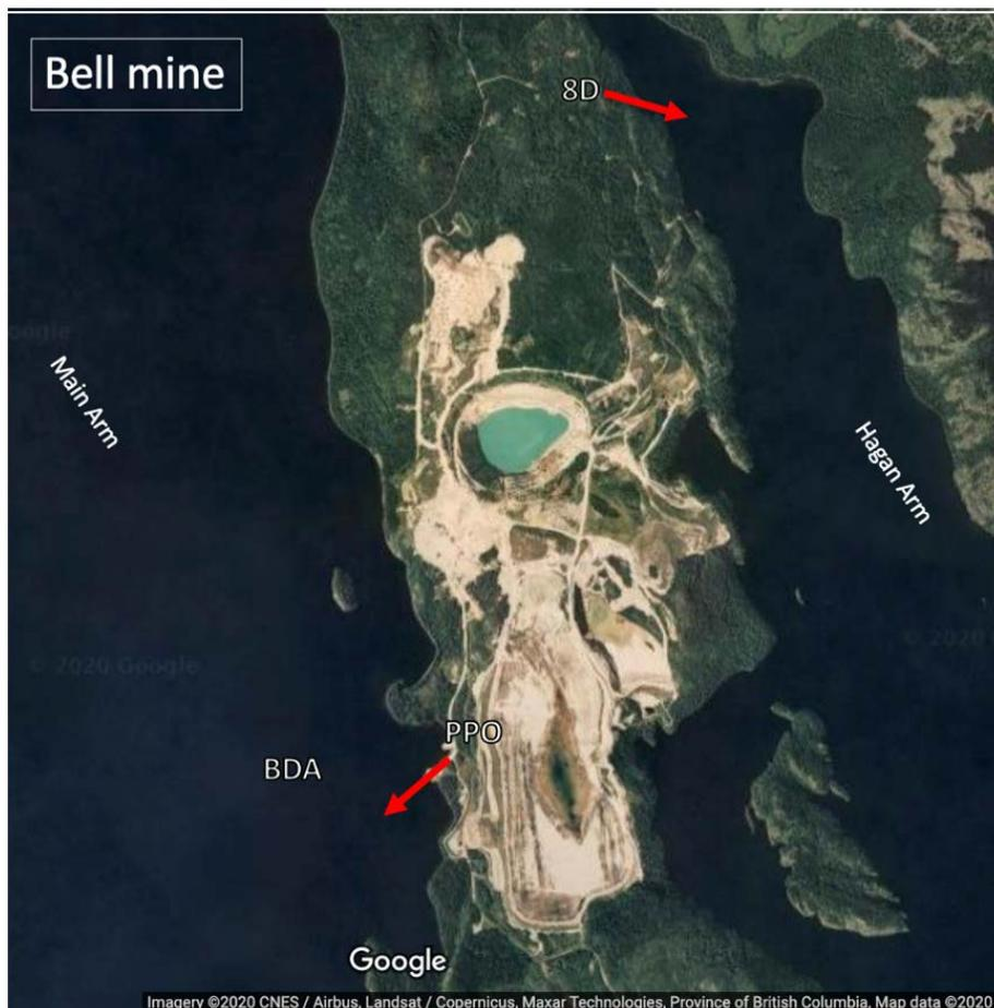
FIGURE 2. MINE-IMPACTED WATER DISCHARGES (RED ARROWS) FROM BELL MINE INTO BABINE LAKE. POLISHING POND OUTFLOW (PPO) IS TREATED WATER THAT ACTIVELY DISCHARGES TO THE BELL DIFFUSER AREA (BDA); 8D DISCHARGE IS UNTREATED WATER THAT PASSIVELY DISCHARGES TO THE NORTH END OF HAGAN ARM.
