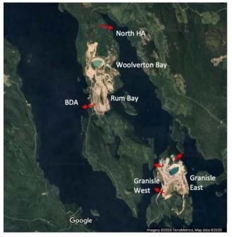
FIGURE 4. RECEIVING AREA SITES IN BABINE LAKE WHERE AQUATIC MONITORING IS PERFORMED: BELL DIFFUSER AREA (BDA); NORTH HAGAN ARM (NORTH HA), WOOLVERTON BAY, AND RUM BAY IN THE HAGAN ARM RECEIVING AREA; AND GRANISLE EAST AND GRANISLE WEST IN THE GRANISLE VICINITY RECEIVING AREA. RED ARROWS INDICATE SOURCES OF CURRENT MINE DISCHARGES INTO BABINE LAKE.
