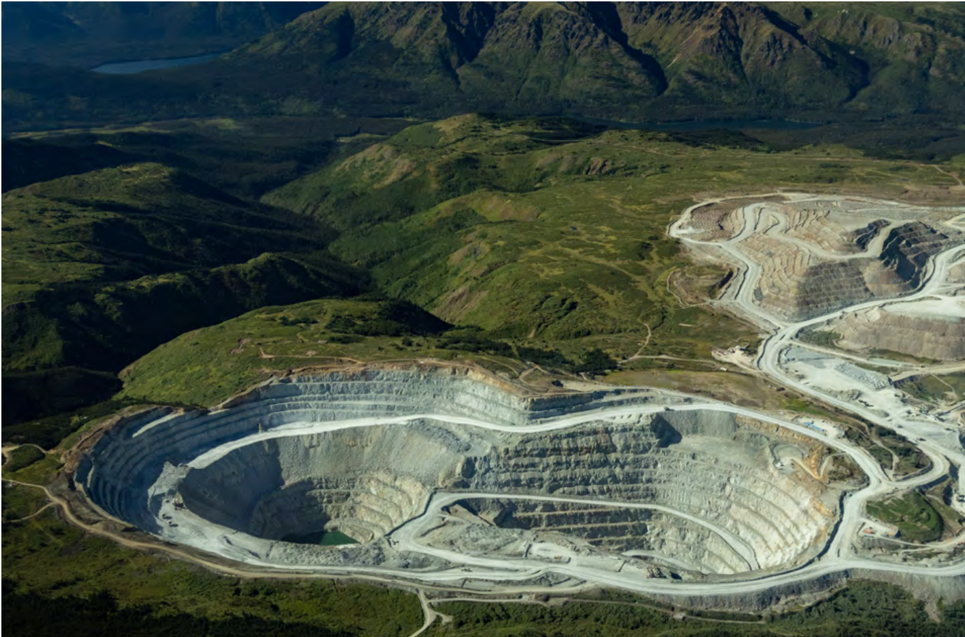
Open pit and waste rock pile at Red Chris Mine with White Rock Canyon Creek drainage and Ealue Lake in background. COLIN ARISMAN | COLINARISMAN.COM
